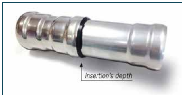
Figure 9 - Check of complete pipe's insertion into the fitting
