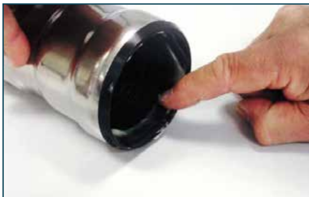
Figure 6 - Internal gasket lubrication
