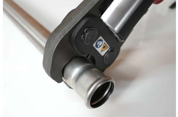
Figure 29 - Making the press connection
