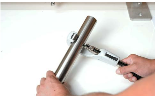
Figure 22 - Cutting the tube to length
