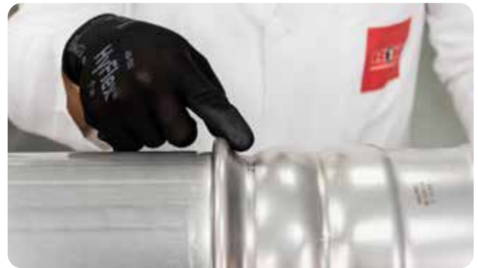
Figure 32 - Visual inspection of oversize pressing
