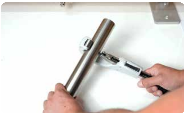
Figure 22 - Cutting the tube to length
