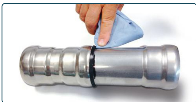
Figure 8 - Cleaning of the grease residual
