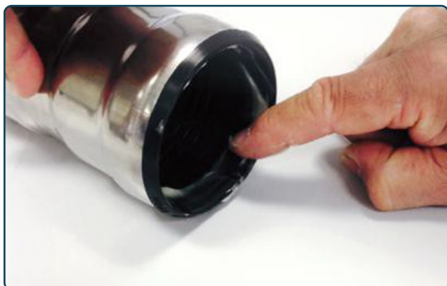
Figure 6 - Internal gasket lubrication
